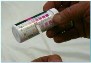
$\mathbf{F}_{igure}$  **50.** Home water-testing kits typically rely on a color change on a test strip to determine the concentration of a contaminant.
