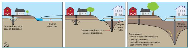
Figure **34.** Overlapping drawdown cones can lower the water table to the point where neighboring homeowner wells and rivers can go dry.
