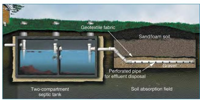
${\bf F}_{igure}$  61. A septic tank and soil absorption field system.
