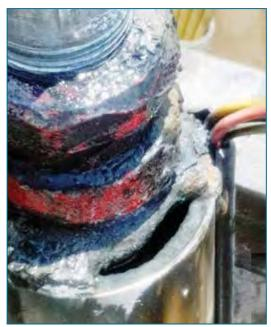
**F**<sub>igure</sub> **35.** Stray electrical currents formed a hole in this submersible pump. Water was forced through the hole in the bottom of the pump, causing the well screen to collapse and the well system to fail. (Source: Mike Prestigiacomo)
