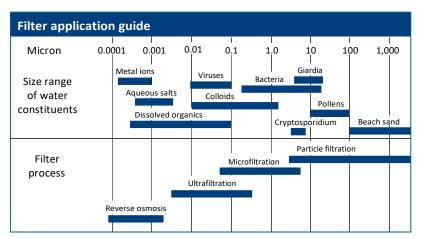
**F**<sub>igure</sub> **52.** A filtration guide showing the appropriate filter processes according to the particulate size of the water contaminant. (Modified from U.S. Bureau of Reclamation, Water Quality Improvement Center).
