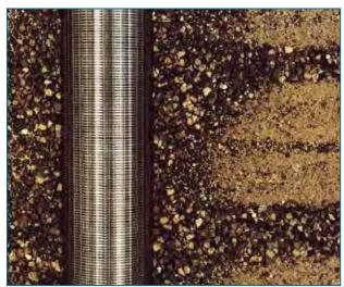
**F**<sub>igure</sub> **31.** Pumping the well has removed fine-grained sediment from around the well screen. Reprinted by permission of Johnson Screens, a Weatherford Company.
