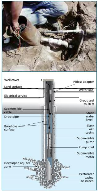
**F**<sub>igure</sub> **32.** A pitless adapter protects pipes from freezing in cold weather. (Source: Gary Hix)
